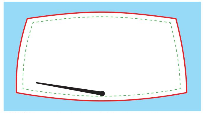
PLEASE NOTE: A curve (smile) needs to be put on the final artwork for most vehicles to counter the curve of the glass. A standard amount is 30mm but each vehicle is different and must be measured. Be mindful of placing logos and text so they don't get covered by wipers or reversing mirrors. Text must be a minimum of 3mm thick - finer than this and it may be difficult to read due to the holes in the material.
